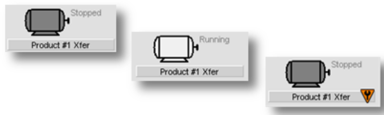
Figure 3: Optimized use of color and icons to indicate status from the PlantPAx library of objects.
