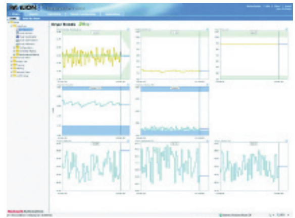
Pavilion8's browser-based user interface provides easy access to monitor all aspects of the MPC solution.
